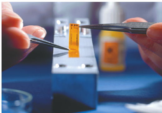
FIGURE 2. You can apply strain gages to a clean, smooth surface using a room-temperature adhesive for short-term tests at room temperatures. For long-term tests or tests at high temperatures, you can use heat-cured adhesives.
